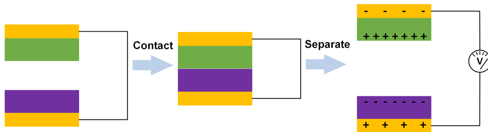
Figure 1.4: Graphic illustration of triboelectric effect.
