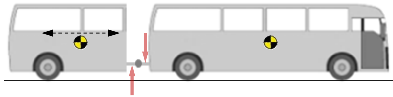
Figure 4.3: Tractor weight distribution affected by the trailers [9]
