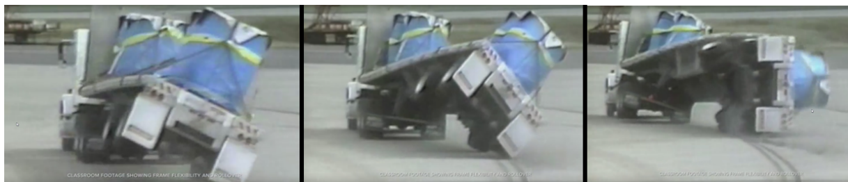
Figure 1.1: Footage of a truck rollover due to excessive speed in a turn [6]
