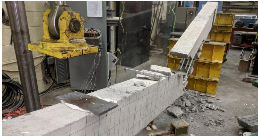
Figure 4.38 – BM 10.5-N: Catastrophic shear failure
