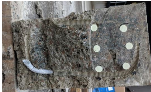
Figure 4.1 – Typical post-failure section at critical shear region
