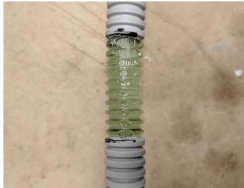
Figure 3.1 – GFRP stirrup with bend protector removed
