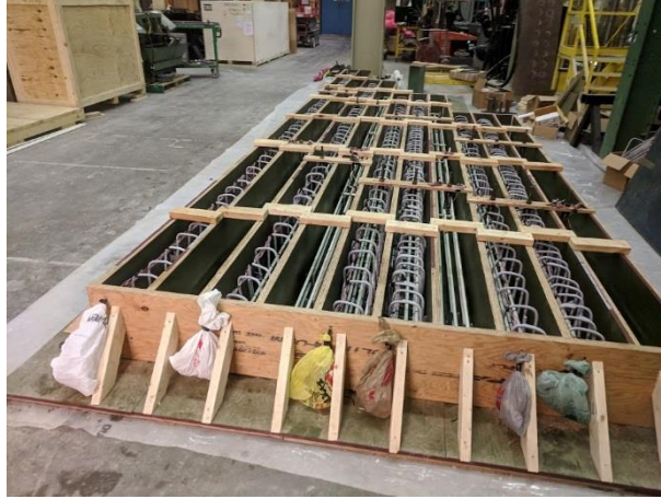
Figure 3.3 – Gang form for specimen casting
