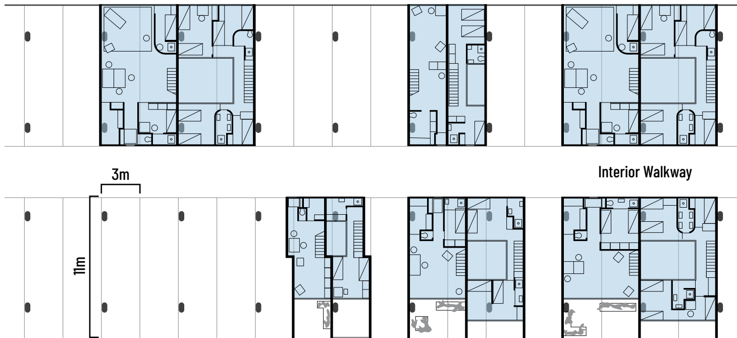
Figure 5.19 Typical plan and cell dimensions of the viaduc, showing potential unit designs.
