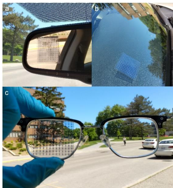
Figure 5-7. A detector array placed a. inside a vehicle, b. on the windshield, c. on glasses.
