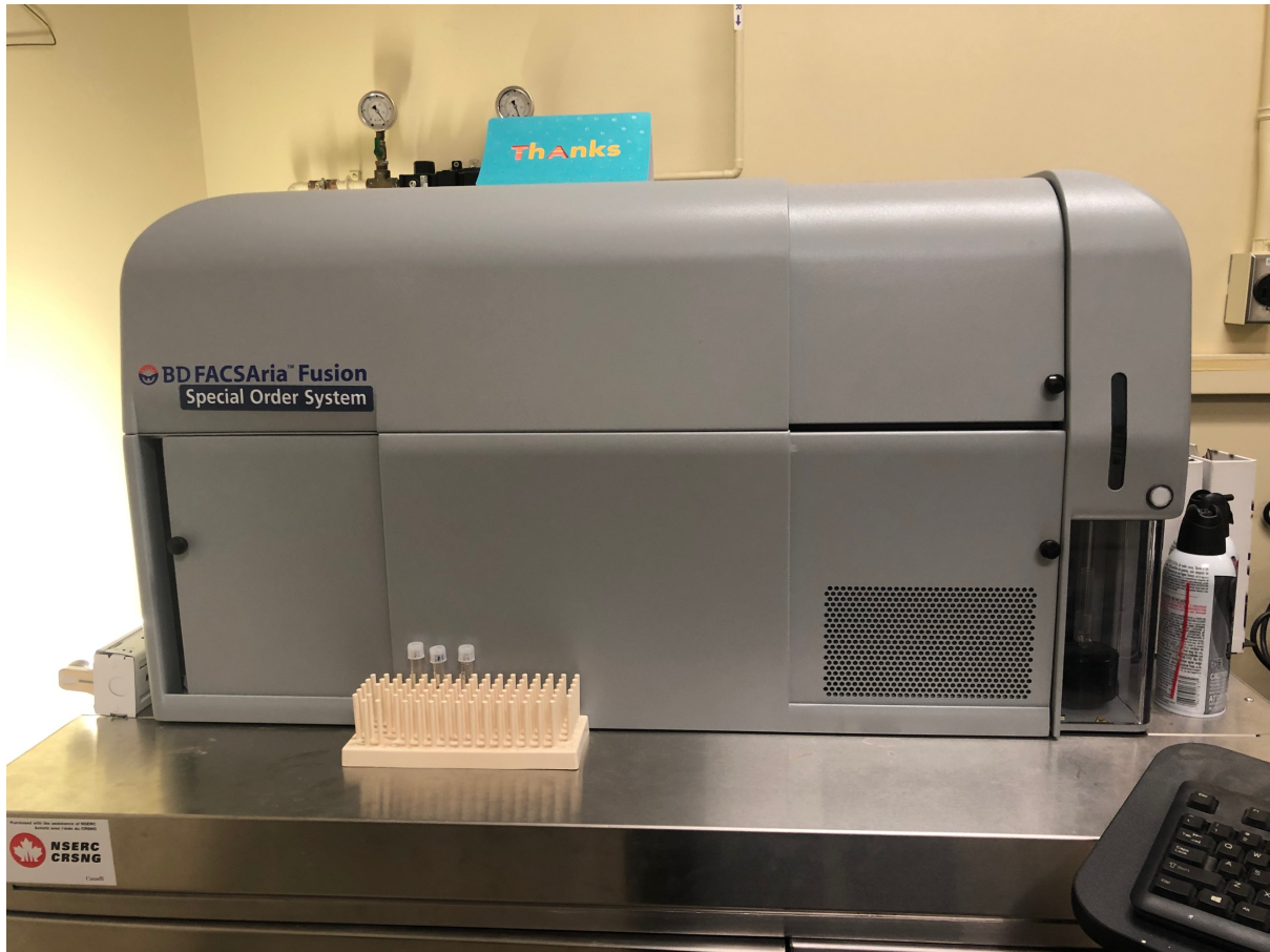
Figure 3.3 Picture of BD FACSAria Fusion Special Order System in the lab from biology department.
