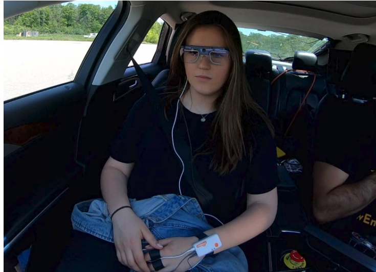
Figure 3.2: A participant sitting in the Autonomoose and set up with the eye-tracker, skin response, and heart rate sensors.
