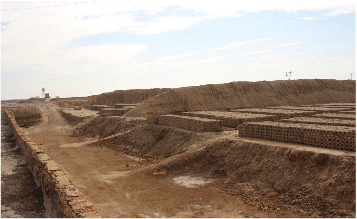
Figure 85 Unfired brick storage around the kiln
