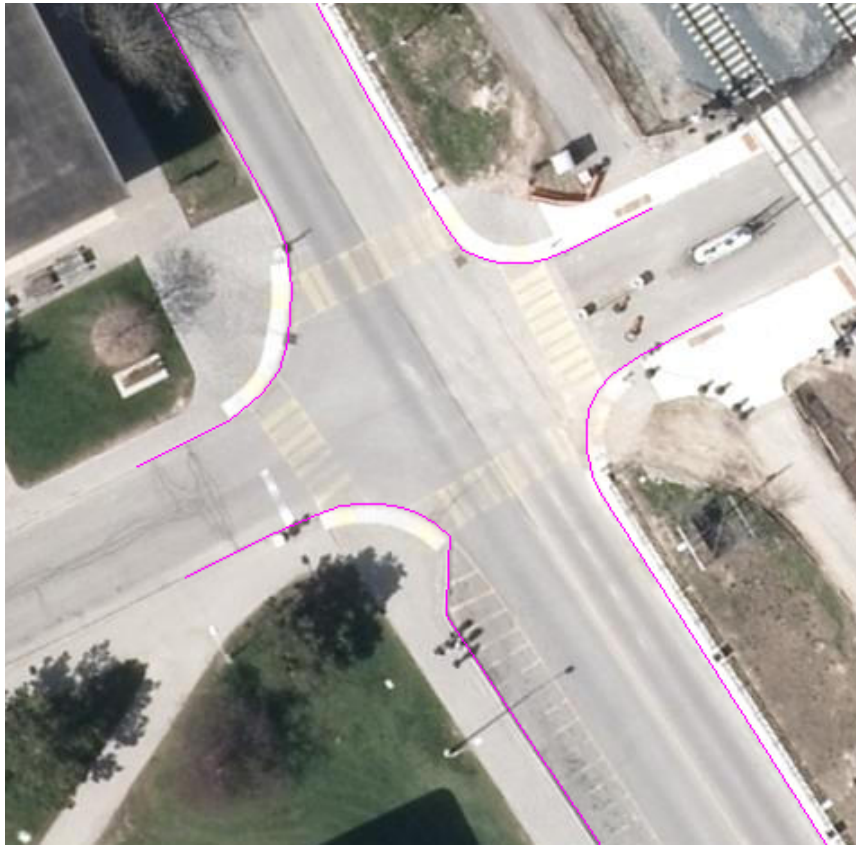
Figure A.4: Curb lines traced in ArcGIS with visible road markings
