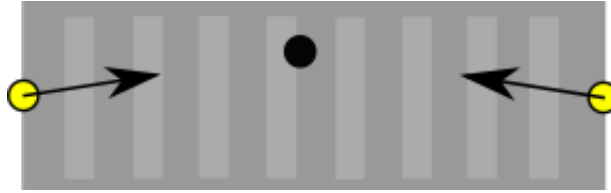
Figure 3.5: Crosswalk with unit vectors (black arrows) pointing from entrance points (yellow) toward pedestrian (black circle)
