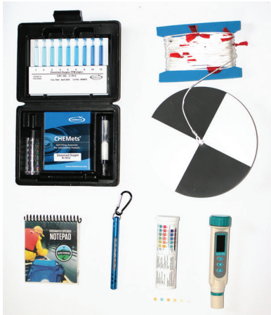
Fig. 205. Tools used for data collection: (1) Dissolved oxygen kit; (2) Secchi Disk; (3) Field Notepad; (4) Stream Thermometre; (5) Test strips; (6) Conductivity meter
