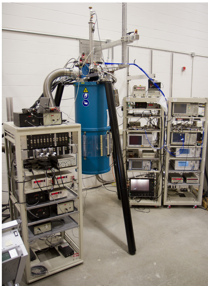
Figure 3.7: Experimental setup. General view of the experimental setup developed in this work with the DC rack on the left of the fridge and two microwave racks on its right. The probe is inserted in the dilution fridge with a device, and the magnetic field compensation system's coil can be seen warped around the blue outer vacuum shield of the unit.
