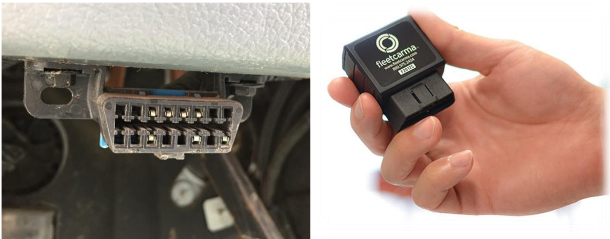
Figure 4.3: The OBD port of a vehicle at the left, and the FleetCarma C2 device at the right side
