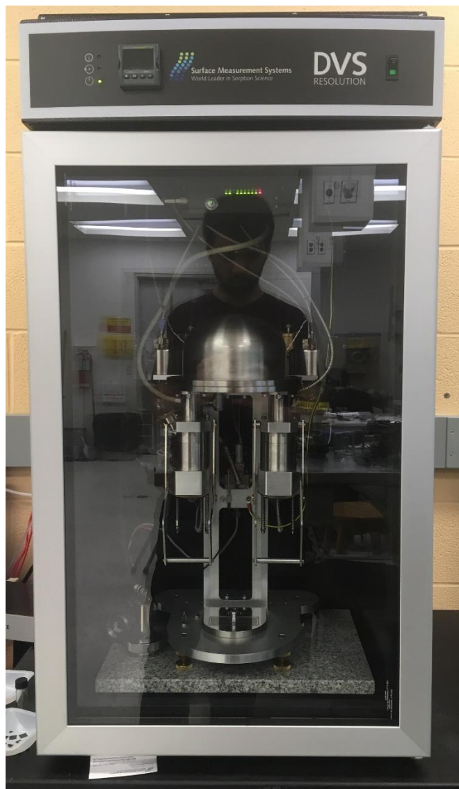
Figure 16: Digital vapor sorption device used to measure specific surface area of fabricated samples
