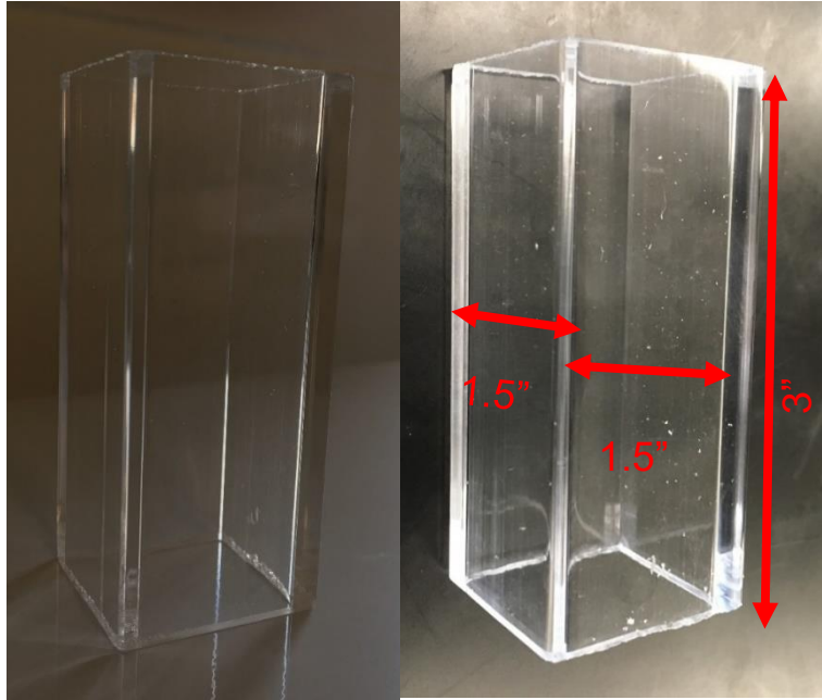
Fig. 5-1: Plexi-glass square tube used for holding the transparent soil
