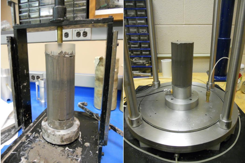
Fig. 7-2:(a) Trimmed soil sample on a pedestal; (b) Sample on the resonant column base platen.
