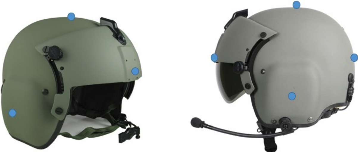
Figure 17: Reflective marker placement on the Gentex HGU-56/P helmet
