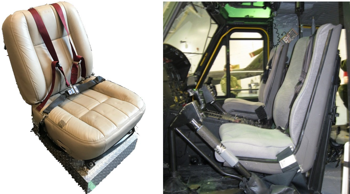
Figure 20: Comparison of study seating vs. real seating. A – Car chair with 4-point harness used in study; B – Pilot seat inside a Griffon Helicopter
