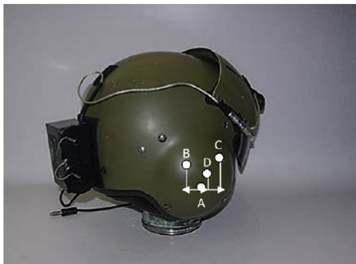
Figure 8: Shift in COM with various helmet configurations. A: the head alone, B: the helmet alone, C: NVGs, D: NVGs and CW. From Forde et al. (2009)
