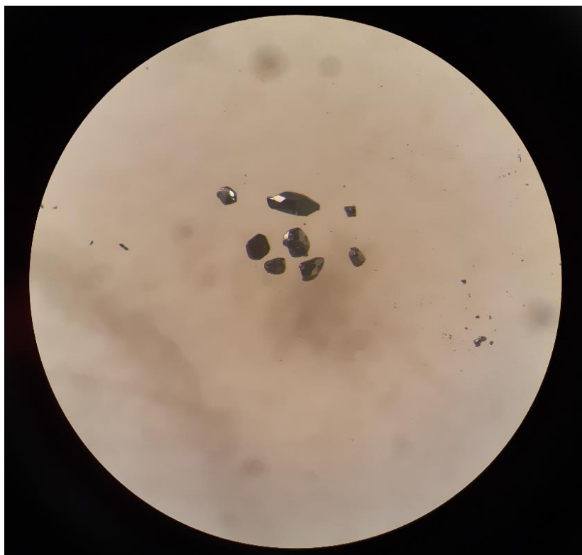
Figure 16. Light microscope image of \alpha\text{-Pb}_2\text{GeSe}_4 crystals grown using a Zn flux.
