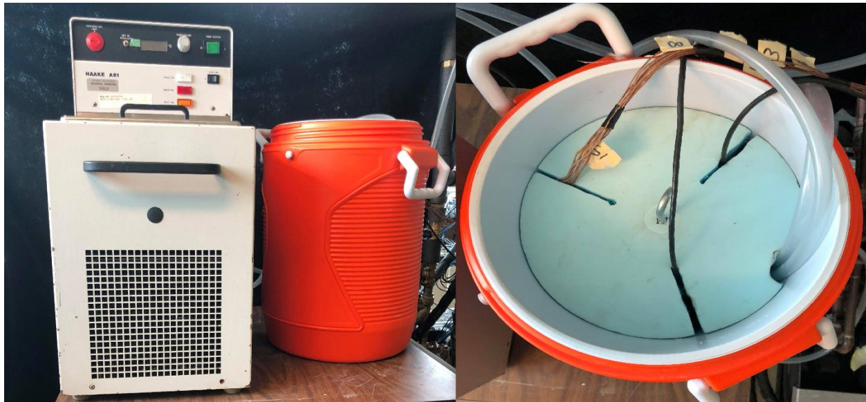
Figure D1: Calibration equipment set-up with RTDs and thermocouples
