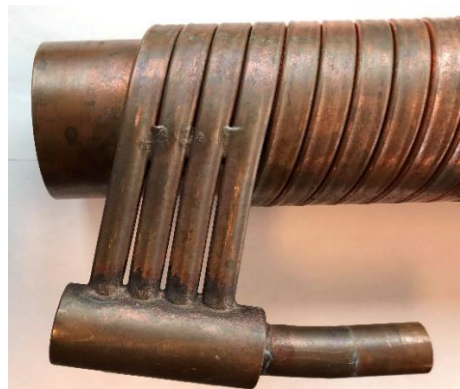
Figure 4-3: Coil set of 4 coils on a random DWHR system
