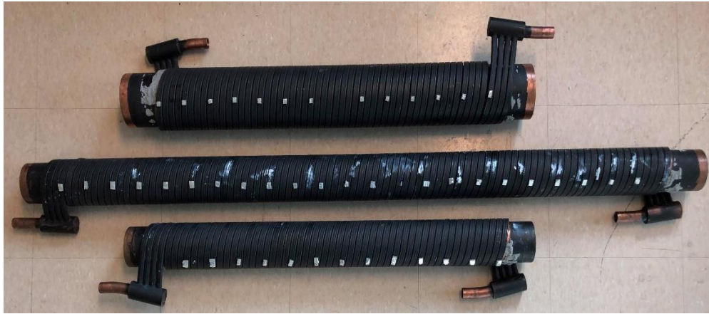
Figure 4-5: Double coated DWHR systems used for infrared thermography
