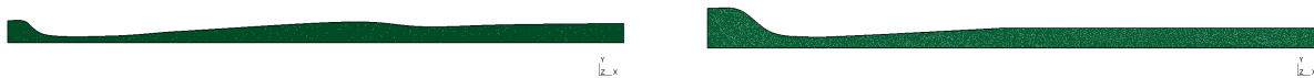
Figure 5.52: A picture of the mouthpiece cup region of the axisymmetric computational trumpet (left) and trombone (right) produced in GMSH used in Section 5.8.2.
