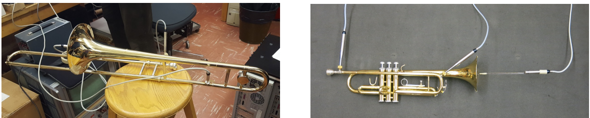
Figure 2.1: Placement of the microphones on the trombone (left) and trumpet (right).
