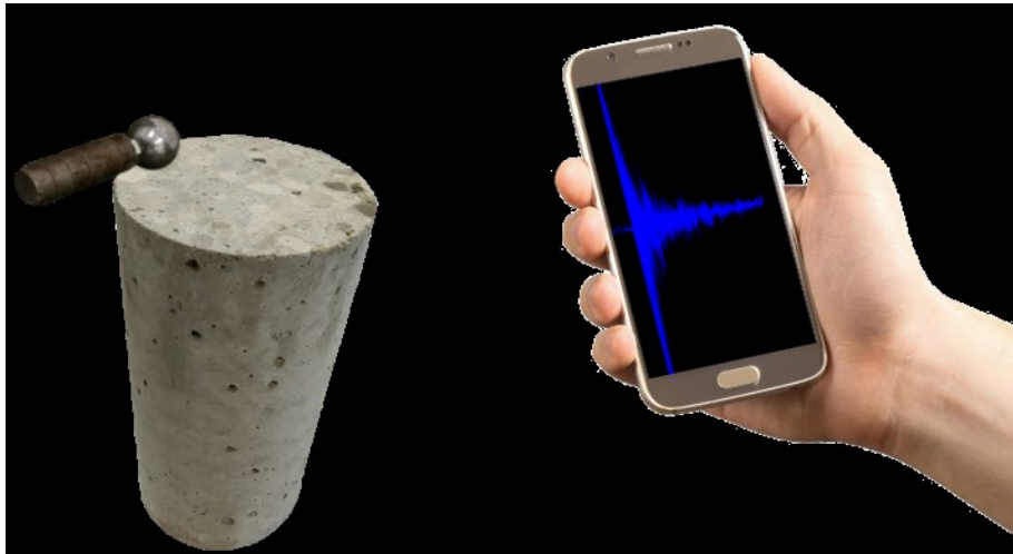
Figure 1.2 Sketch of final dynamic test methodology proposed, in order to make the test more affordable, time-efficient, and portable.
