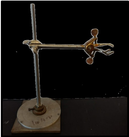
Figure 5.10 Retort stand used to hold the smartphone at a constant close distance from the specimen during the resonant tests
