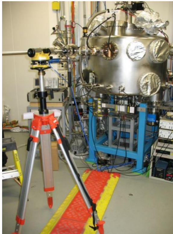
Figure 4.1: Incident beam is roughly aligned with a telescope through windows of UHV chamber
