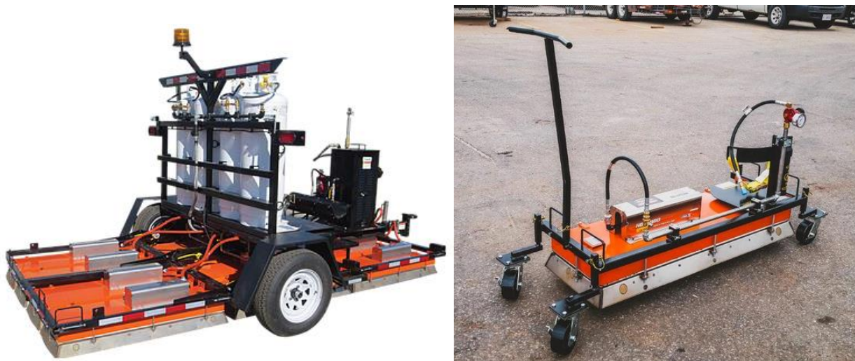
Figure 3.8: Infrared Heating Patchers. Left – 8.6’ by 6.6’, Right – 20” by 51” (Heat Design Equipment Inc. 2019)
