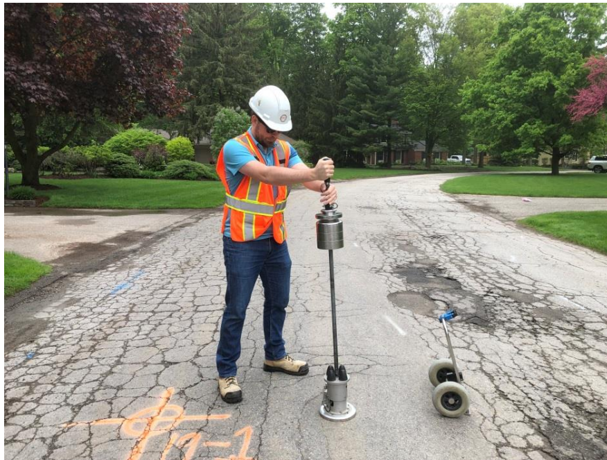
Figure 4.8: Lightweight Deflectometer Testing at Location #3 on Sugarbush Drive, Taken May 30 th , 2019
