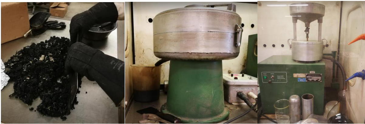
Figure 4.20: Left - Sample Separating, Centre – Centrifuge, Right – Fine Materials Centrifuge
