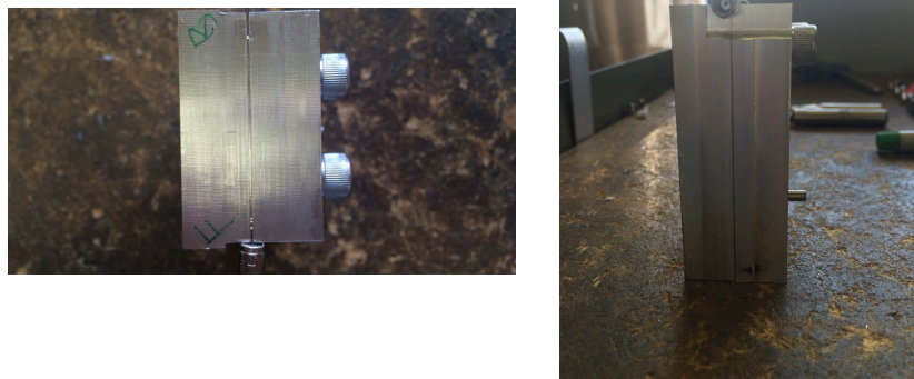
Figure 2.6 Aluminum jig used to open the trapping capillaries
