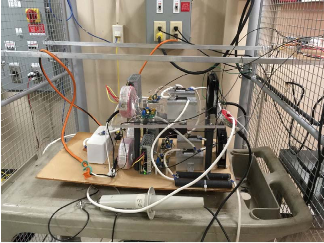
Figure 2-18: High-voltage full-bridge square/PWM generator.
