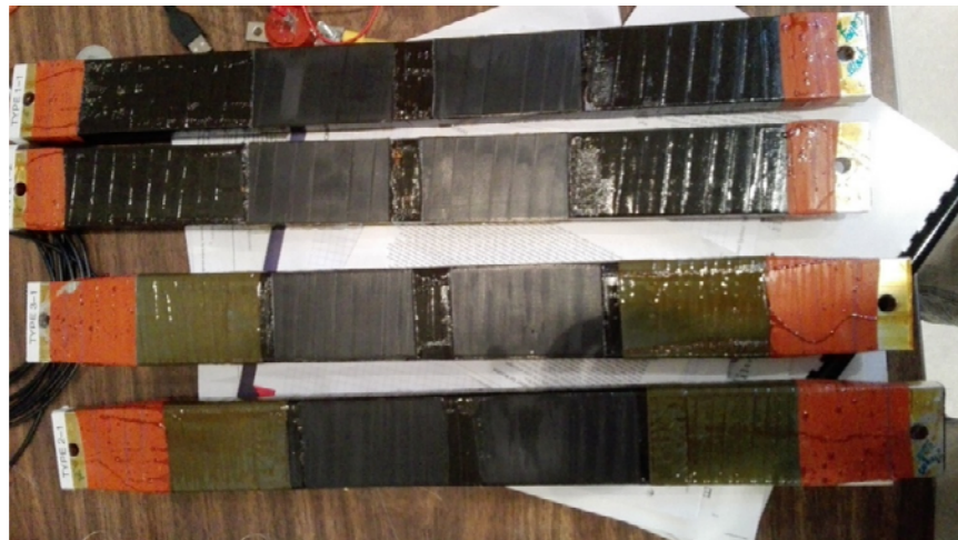
Figure 2-2: Photograph of samples prepared for conductivity measurements (courtesy of General Electric Power Conversion of Canada, Peterborough, Ontario).
