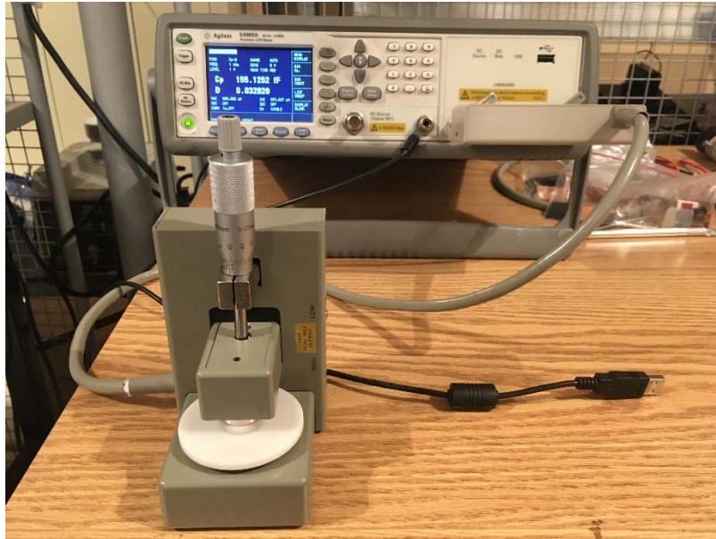
Figure 2-9: The setup used for relative permittivity measurement.
