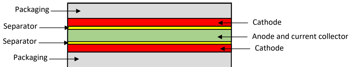
Figure 13: Zinc-air battery cell configuration.
