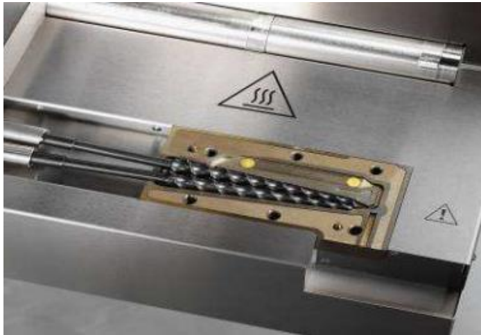
Figure 3.5 Co-rotating conical twin-screw extruder configuration
