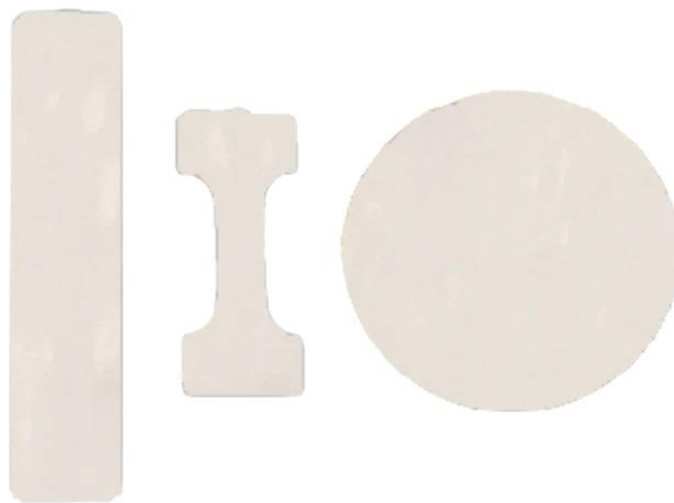
Figure 3.3 Flexural / IZOD impact (left, rectangular), tensile (centre, dumbbell) and Gardner impact (right, circular) specimens for mechanical characterizations
