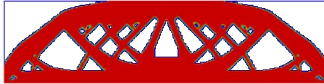
Figure 2.13. Topology optimization result of the MBB beam problem with 45 deg overhang constraint [146].
