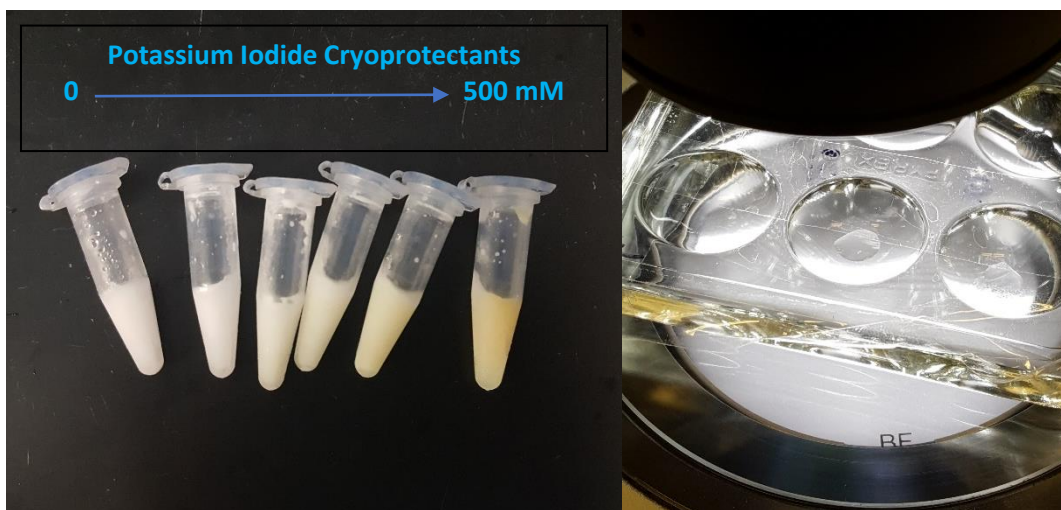
Figure 18: Iodide soaking of WT rcPEPCK crystals. Cryoprotectants (left) contained a solution identical to the reservoir solution of the crystals, with the addition of PEG 400 and potassium iodide (0-500 mM). Crystals were incubated with cryoprotectant (right) before flash cooling in liquid N 2 .
