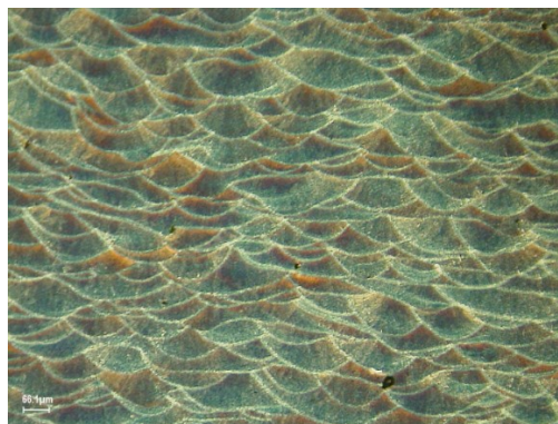
Figure 2-5: Optical micrograph of AlSi10Mg processed by LPBF, side cross-section
