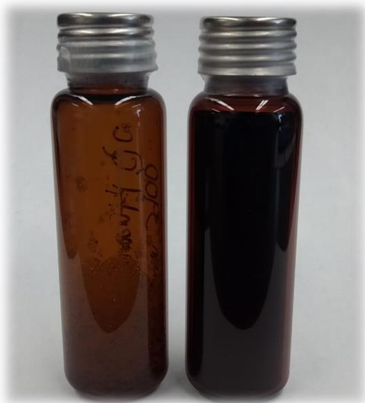
Figure 4.1. Gas generating vial: silicon diffusion pump oil and PS/DVB particles (Left) and carbon fiber mesh coated with the PDMS/HLB (Right).
