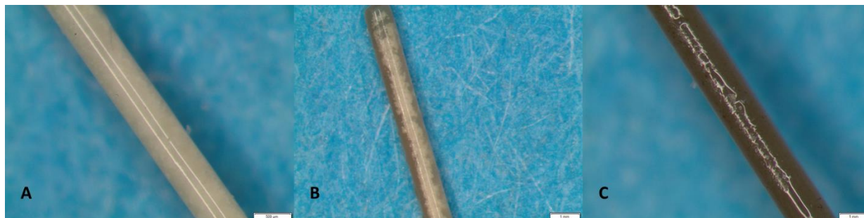
Figure 2.5. Microscopic pictures of a PDMS/DVB overcoated fiber used in avocado extraction. A. PDMS overcoated fiber prior to avocado extraction (3.2X magnification). B. PDMS overcoated
