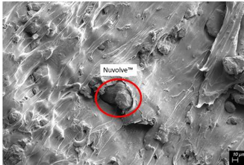
Figure 3.3-14: SEM micrograph of 30B/0 (untreated) at 250x magnification
