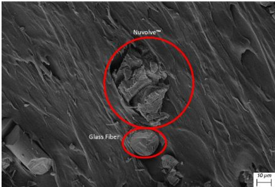
Figure 3.3-16: SEM micrograph of 15B/15 at 2000x magnification
