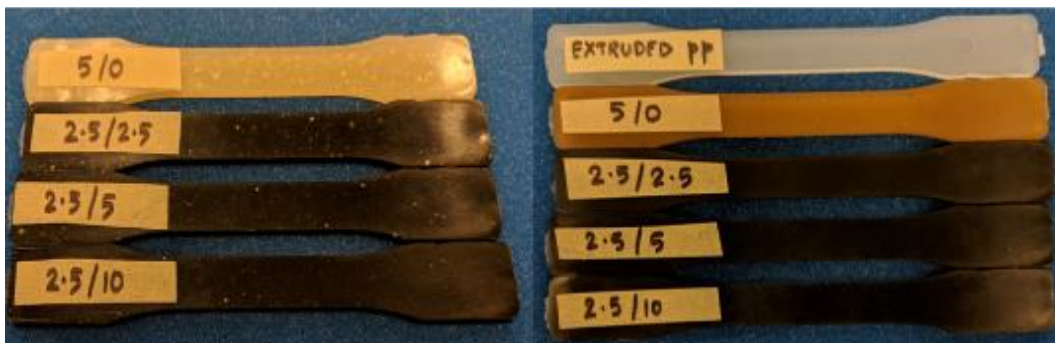
Figure 4.2-2: Visual presentation of ASTM D638-10 dogbones of the composite; CNF (left) and CNC (right)
