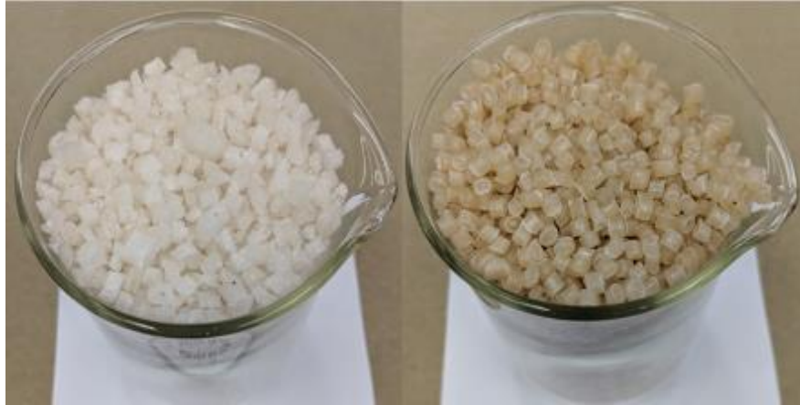
Figure 4.2-1: Nanocellulose 5% masterbatch with PP; CNF (left) and CNC (right)
