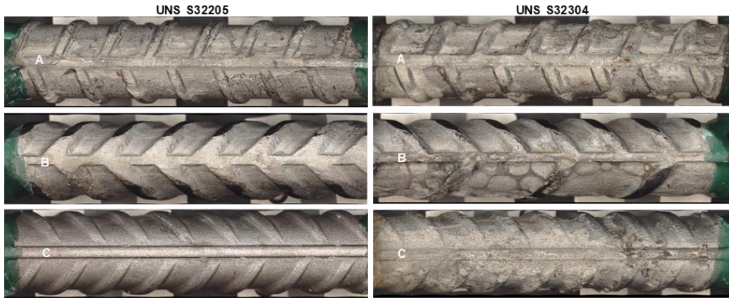
Figure 8-11. Corroded UNS S32205 and UNS S32304 bars after pickling the samples to remove corrosion products. These bars are the same as those shown in Figure 8-3.
