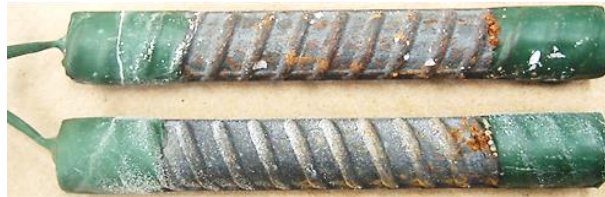
Figure 5-4. An example of before and after testing for pitting potential is shown at the top of the figure. The after tested bar showed clear pitting corrosion underneath the side rib with no crevice corrosion underneath the lacquer. Bars at the bottom, tested for similar purpose but showed crevice corrosion, albeit pitting corrosion in some case, were discarded.
