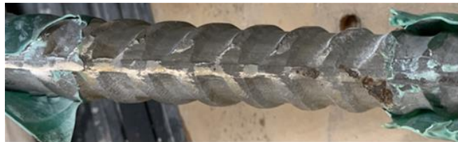
Figure 7-6. The 24100 rebar shown in Figure 7-5 with the area underneath the lacquer exposed to show the absence of crevice corrosion.
