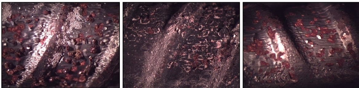
Figure 4.2-20: Corrosion on specimens in (L to R) the tri-hydroxide(NaCl), SEPS with CaCl 2 and in the ASTM solution (NaCl) before pickling
