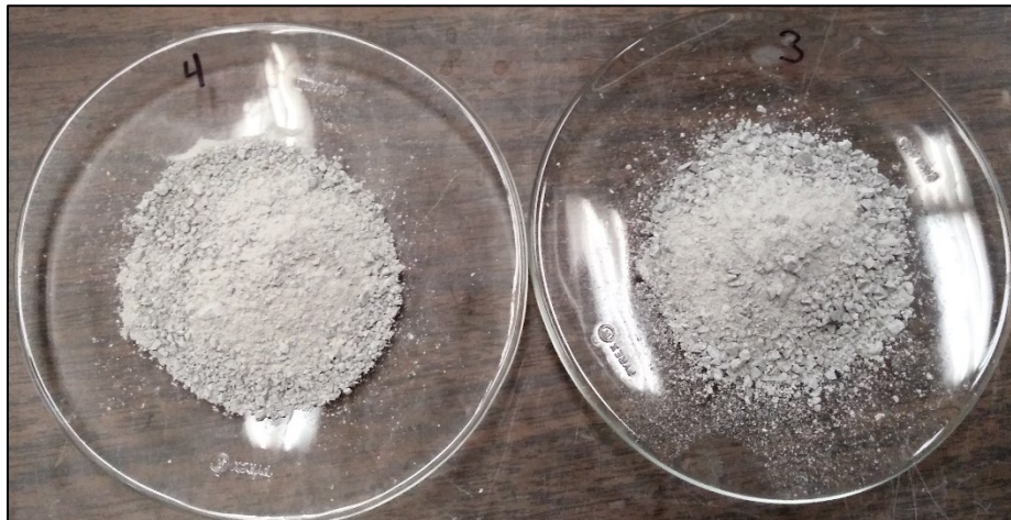
Figure 3.3-2: Cement powder prepared for moisture content testing
