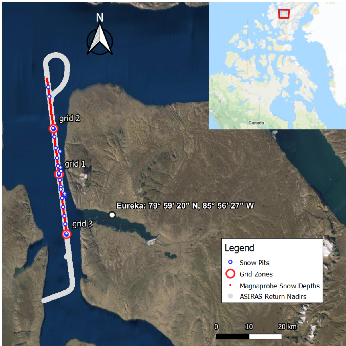
Figure 3.1: Study area map showing dataset locations. ASIRAS returns collected by the Twin Otter flight are in light grey. Snow depth observations collected by ECCC magnaprobes are in red and snow pits in blue. The research and weather station at Eureka, Nunavut is approximately 13 km West of the flight path.
