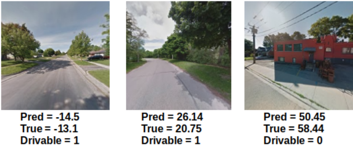
Figure 4.3: Vehicle heading angle ( ^{\circ} ) prediction result and drivable classification.
