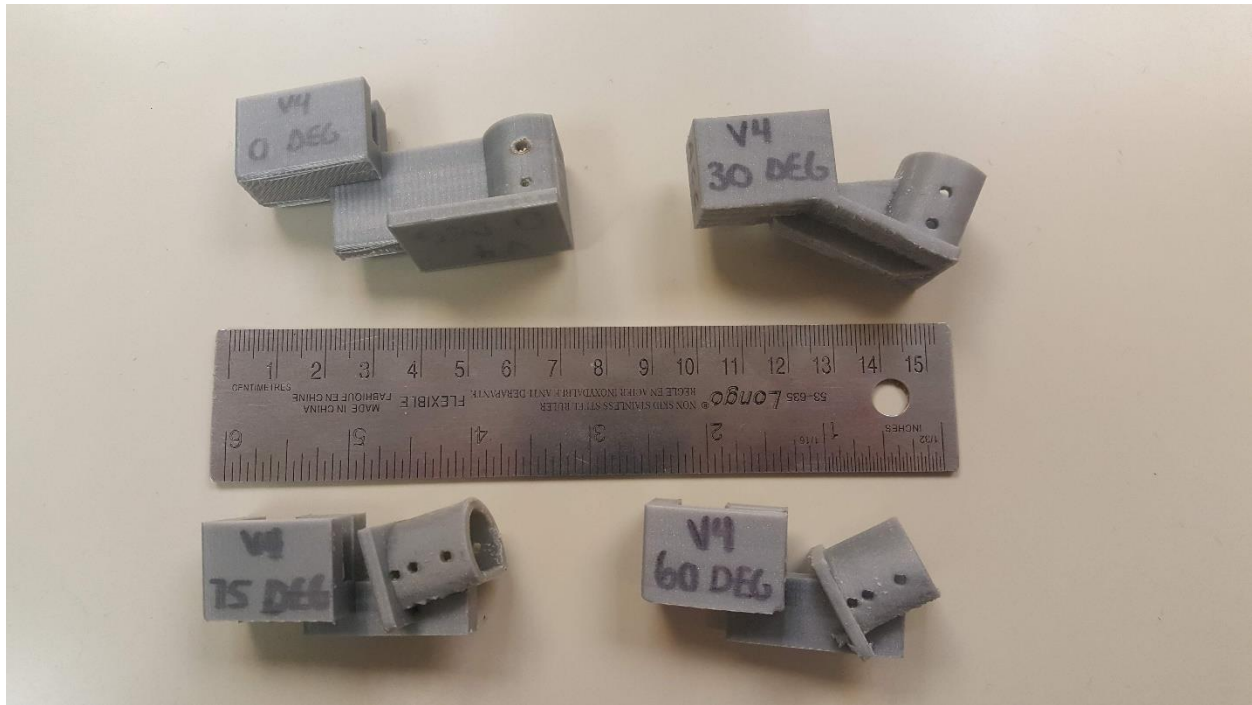
Figure 25. Mounting pots generated differing glenohumeral angles. The rectangular portion attached to the displacement arm of the testing system, while the cylindrical portion housed the scapula.
