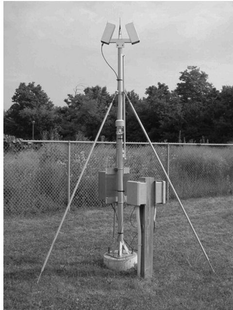
Figure 1.2: The figure shows a representative POSS instrument set up at Egbert station-Ontario. It is a bistatic system with a separate signal transmitter and receiver mounted at an angle from the vertical (Sheppard and Joe, 2008).
