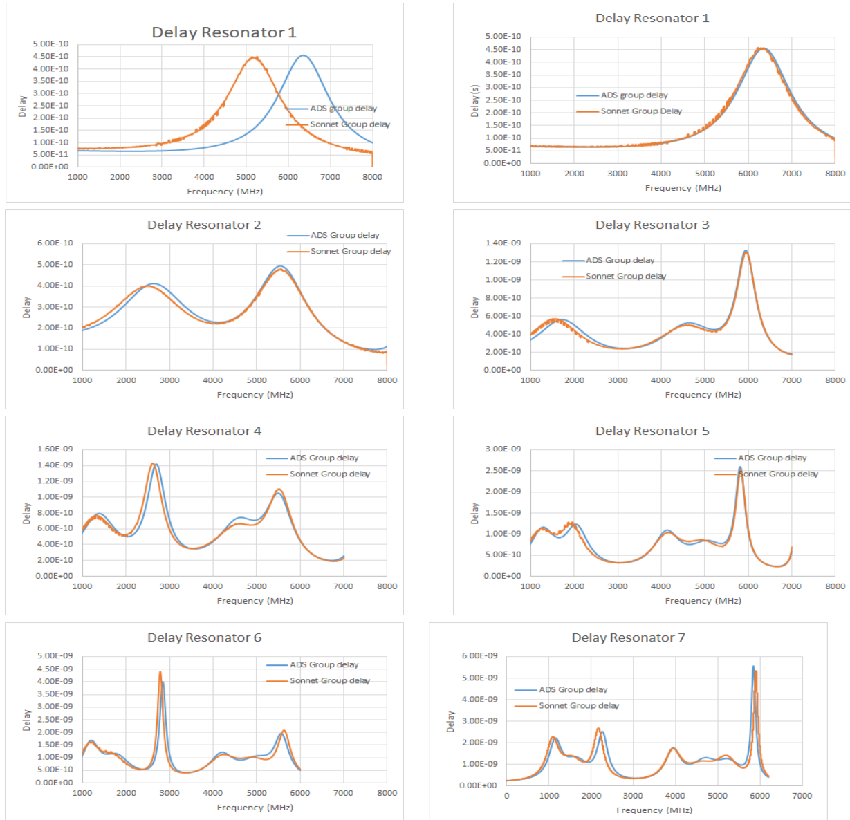
Figure 4.9: The results obtained from group delay optimization using Ness method after incorporating each resonators
