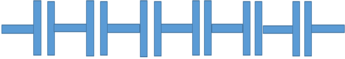
Figure 4.1: Layout of the narrow band 5 pole filter
