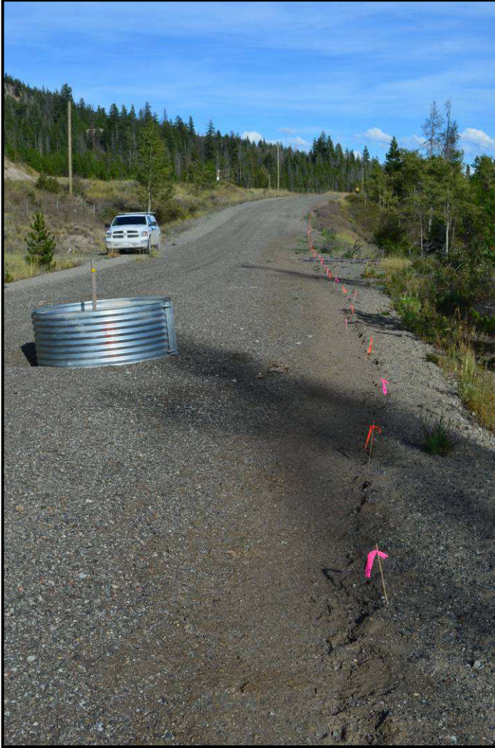
Figure 2.6 The survey line passing by the JA-16-001 borehole (marked by planted wooden stake and surrounded by wide protective metal casing). The pink flags mark the locations of the geophone receivers while the orange ones mark the locations of deployment of the hammer-drop source.
