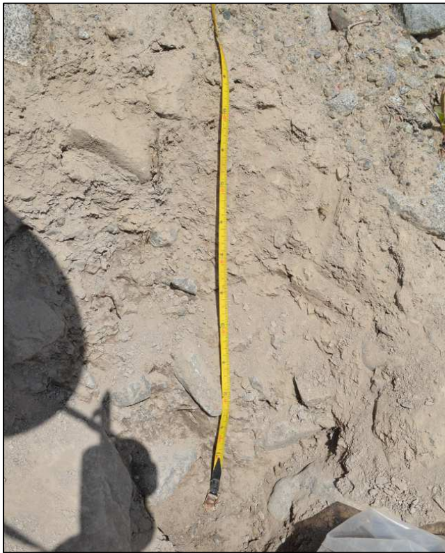
Figure A.10 Stiff, clast-rich till with clay matrix at roadcut FL-8.
