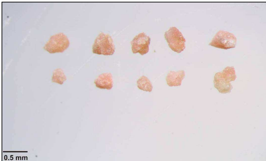
Figure C.3 Mn-epidote grains from the 0.25-0.5mm fraction from sample AR-16-033 belonging to core VTH2014-03.
