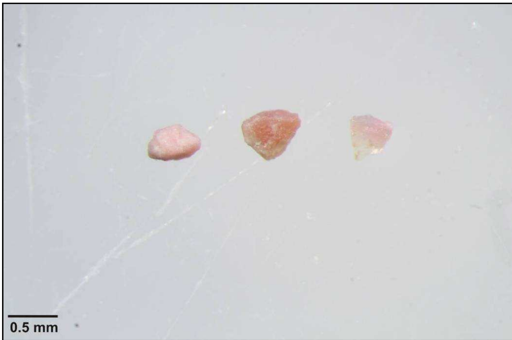
Figure C.17 Mn-epidote grains from the 0.25-0.5mm fraction from sample AR-16-075 belonging to core VTH2014-10.
