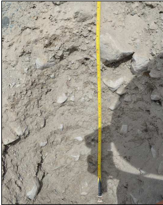
Figure A.3 Stiff, clast-rich till with silt matrix at roadcut FL-5.
