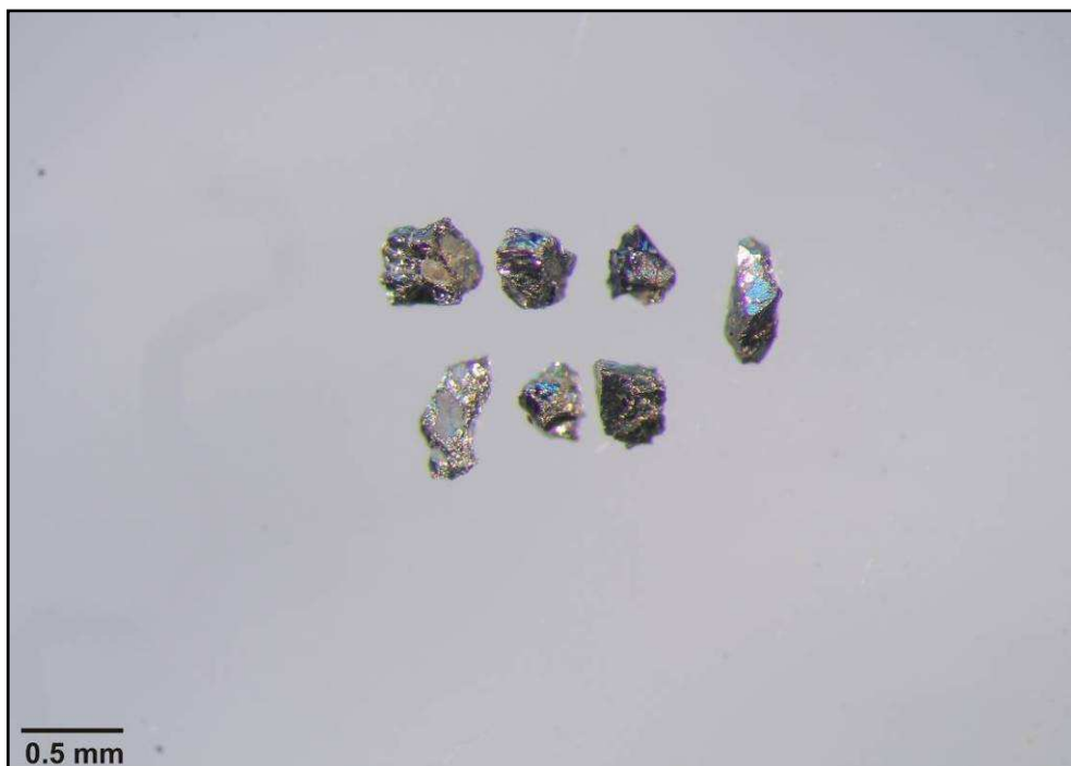
Figure C.14 Pyrite grains from the 0.25-0.5mm fraction from sample AR-16-065 belonging to core VTH2014-10.
