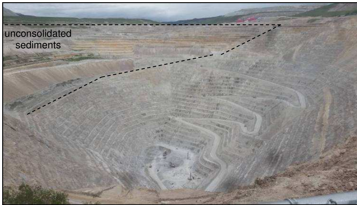
Figure 1.4 View of one of the open pits (Valley) at the Highland Valley Copper Mine, viewed towards the southeast. The thick (~200m in this photo) layer of unconsolidated sediments is shown.
