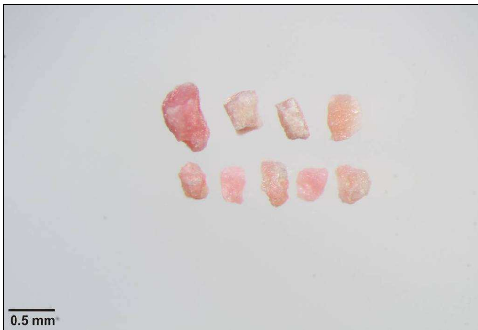
Figure C.13 Mn-epidote grains from the 0.25-0.5mm fraction from sample AR-16-095 belonging to core VTH2014-10.
