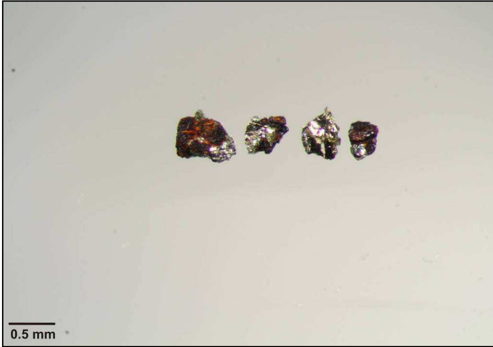
Figure C.49 Chalcopyrite grains from the 0.25-0.5mm fraction from sample AR-16-116 from the Highmont pit.
