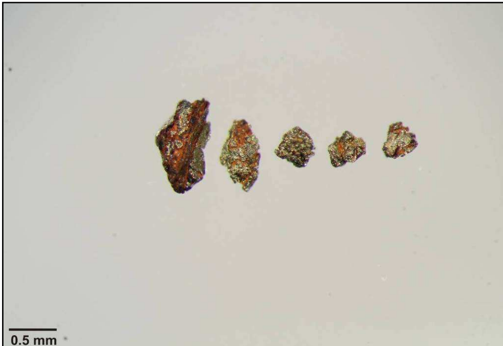
Figure C.29 Chalcopyrite grains from the 0.25-0.5mm fraction from sample AR-16-202 belonging to core VTH2014-13A.
