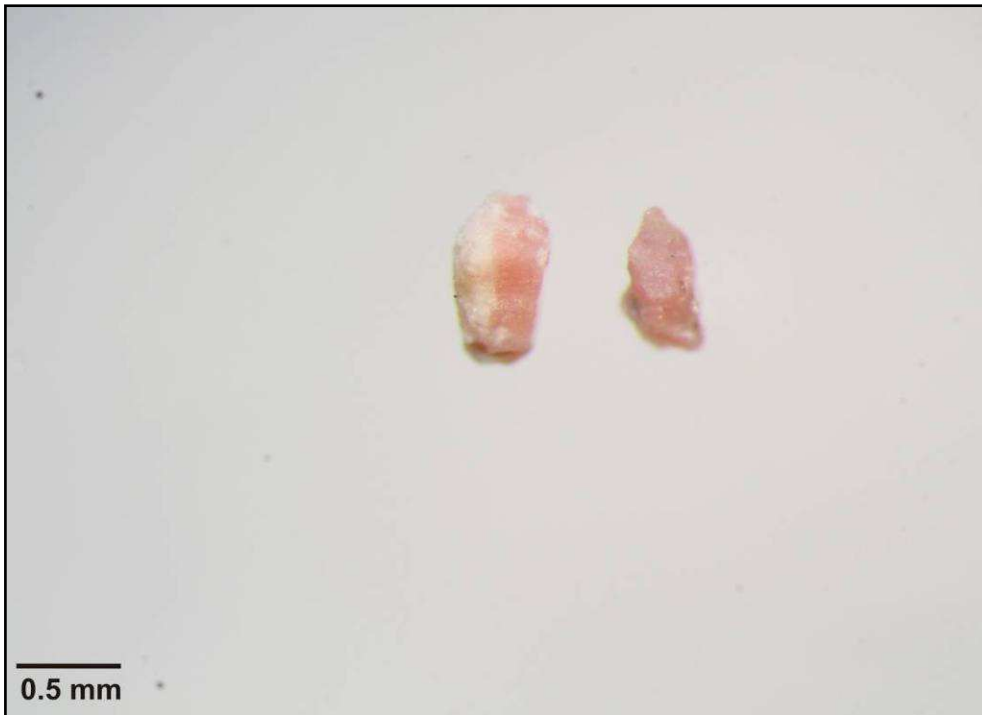
Figure C.27 Mn-epidote grains from the 0.25-0.5mm fraction from sample AR-16-229 belonging to core VTH2014-11.
