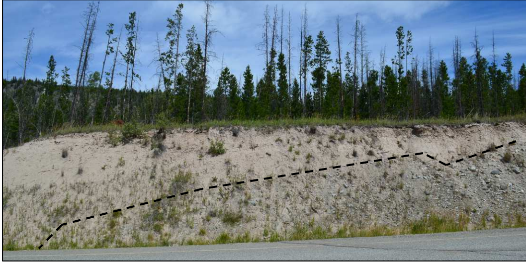
Figure A.6 Fine sand unit overlying till at roadcut FL-6, with the contact between the two shown as a dashed line.
