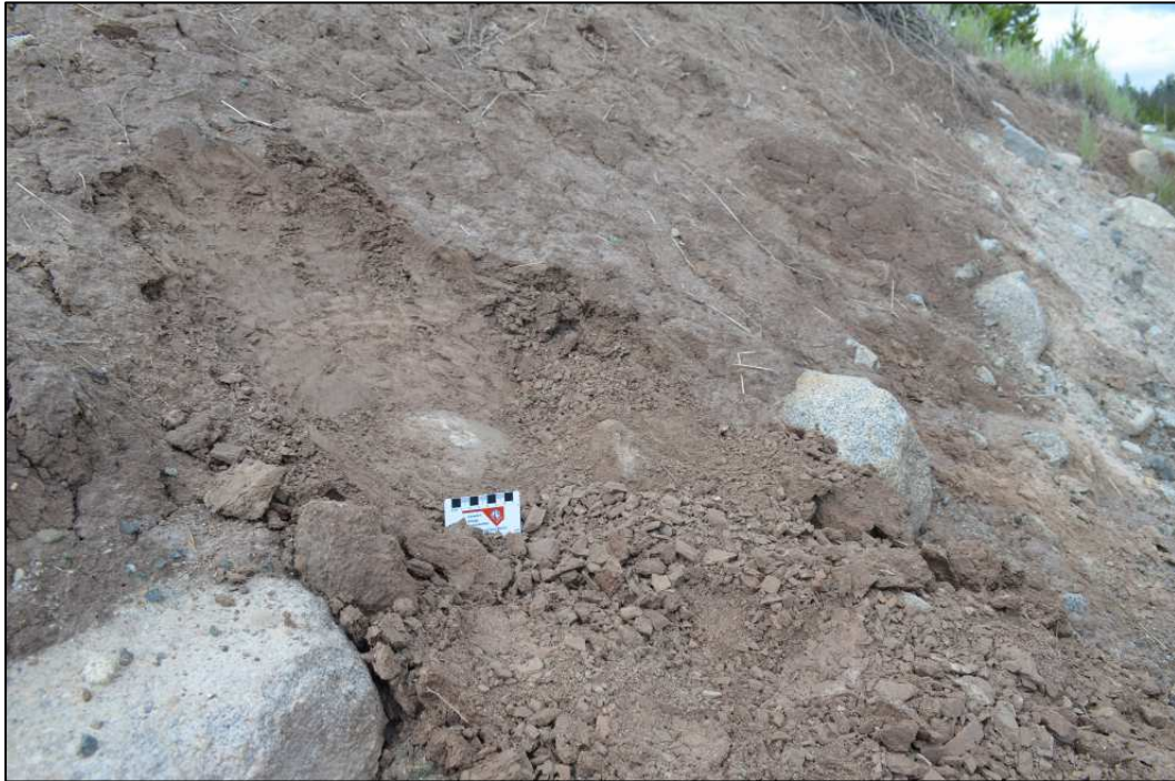
Figure A.11 Laminated silt overlying till at roadcut FL-9.
