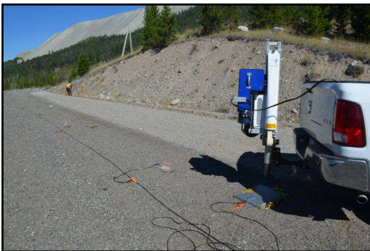
Figure 2.5 The hammer drop system, metal plate and line of receivers of the reflection seismic survey done over the J.A. target.
