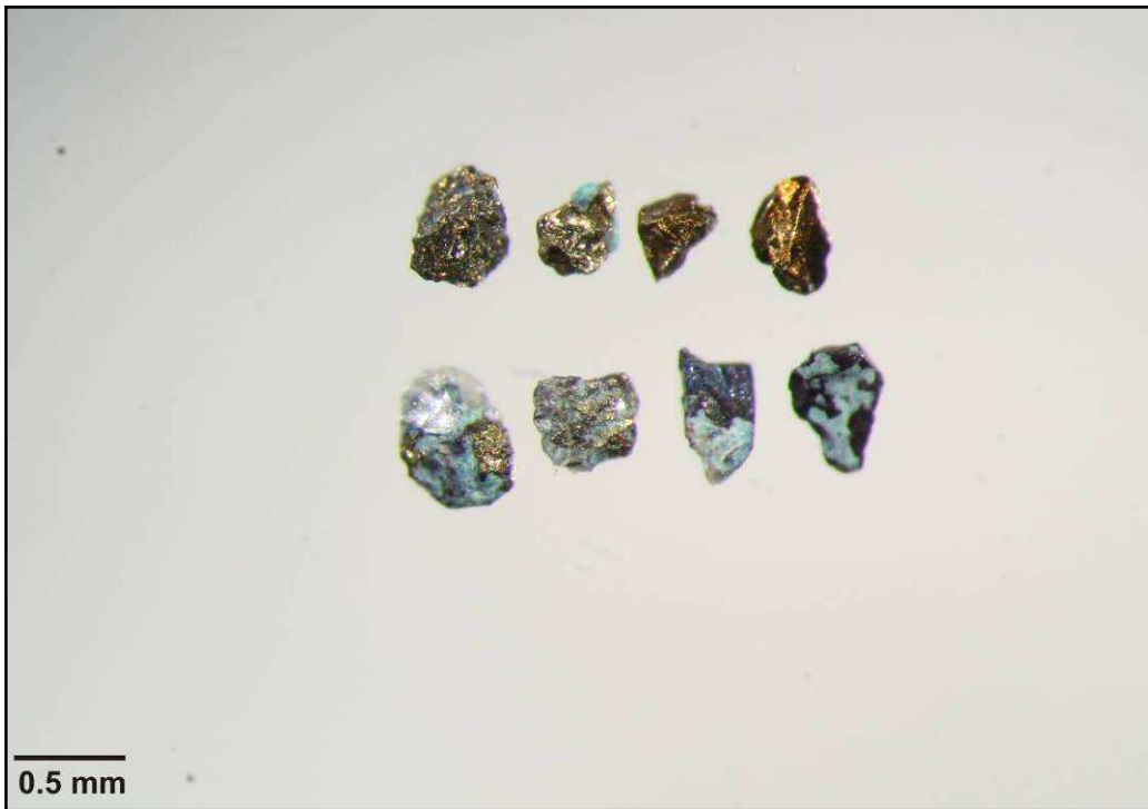
Figure C.25 Chalcopyrite grains from the 0.25-0.5mm fraction from sample AR-16-224 belonging to core VTH2014-11.
