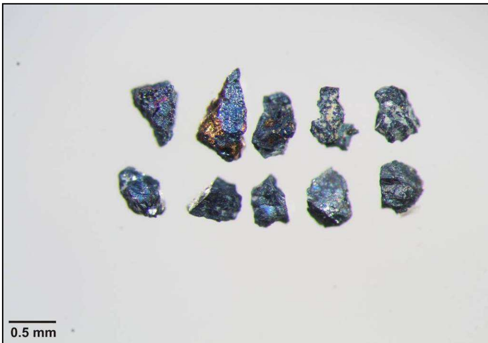
Figure C.35 Covellite grains from the 0.25-0.5mm fraction from sample AR-16-290 belonging to core JA16-001.
