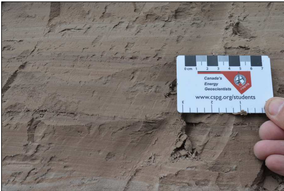
Figure A.9 Top of figure 36; planar laminated silt at roadcut FL-7.
