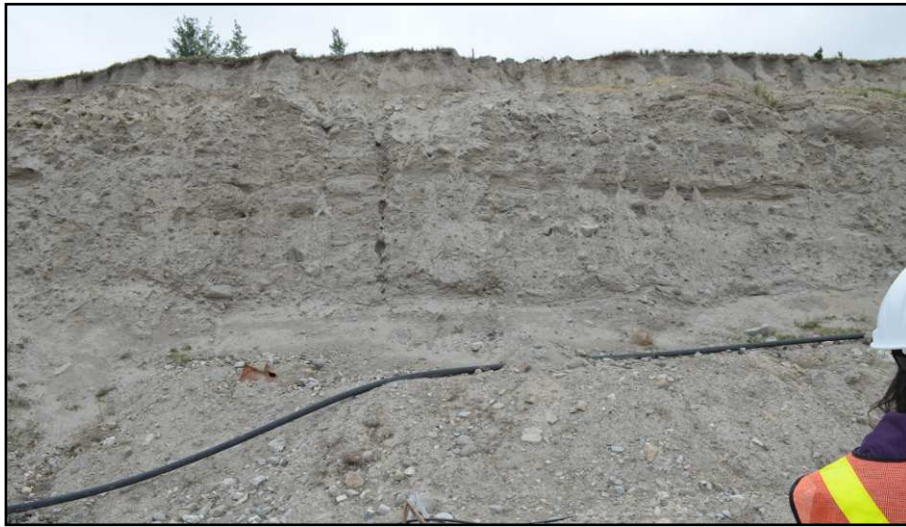
Figure 3.21 Section at location VP-1 on the northeast wall of the Valley Pit. Photo faces northeast. A stiff, poorly-sorted debris flow and thin outwash bed of laminated sand and/or silt are observed.
