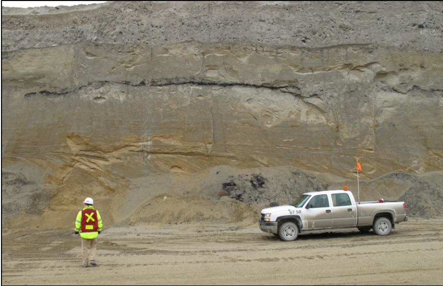
Figure A.18 Deltaic foresets of delta unit dipping to the southeast observed by Alain Plouffe in the Valley pit at station 11PMA050. See figure 6.1b for location.
