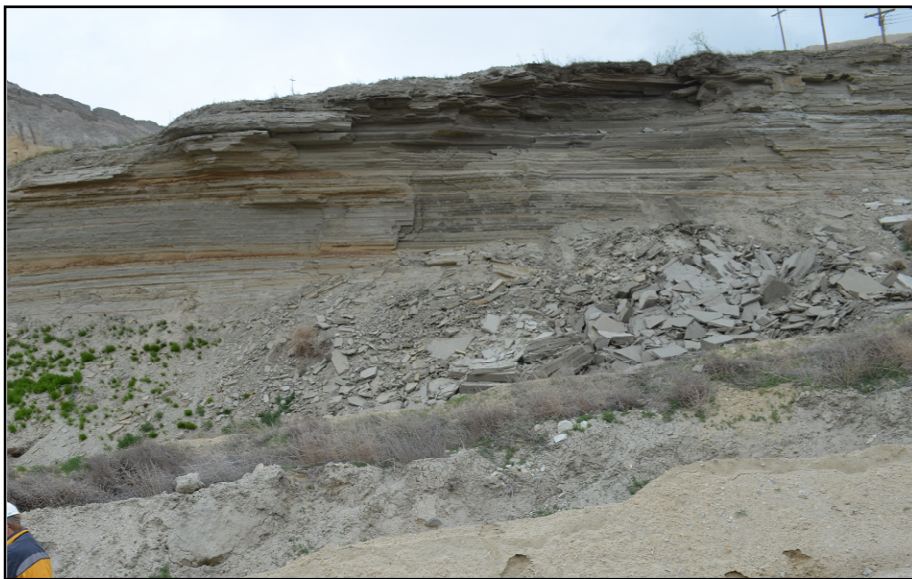
Figure 3.26 Section at location VP-6 on the north wall of the Valley Pit, where laminated, clay, silt and fine sand with organics are present. Photo faces northeast.
