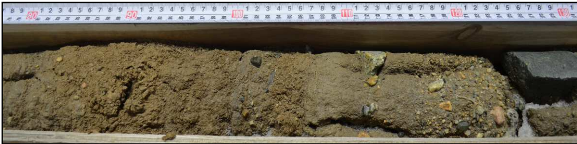
Figure 3.9 Core VTH2014-09 at an elevation of 1207.9 to 1207.4m, showing textural layering and clast gradation forming a distinct interbed within a diamicton sub-unit.
