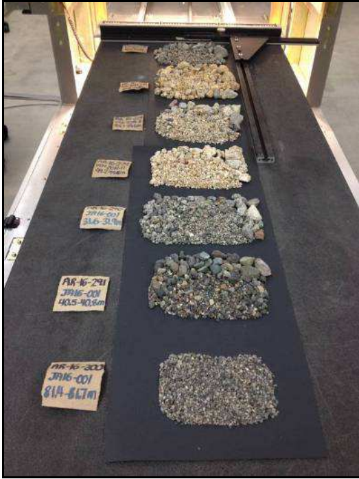
Figure 2.12 The >2mm granule and pebble fraction of selected samples laid out in preparation for hyperspectral analysis.
