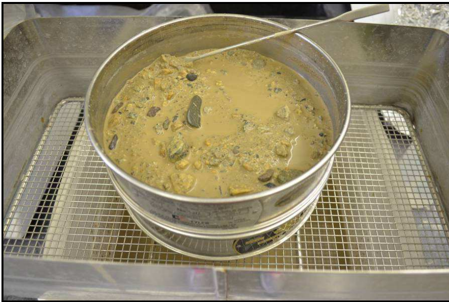
Figure 2.9 Wet sieving a sample using 0.125mm and 0.063mm sieves.
