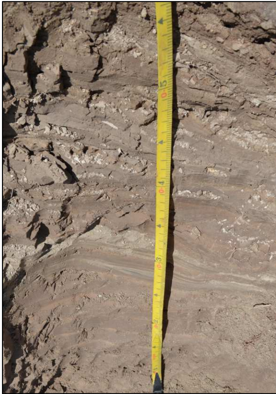
Figure A.12 Stiff clay with fine sand lenses at roadcut FL-10.
