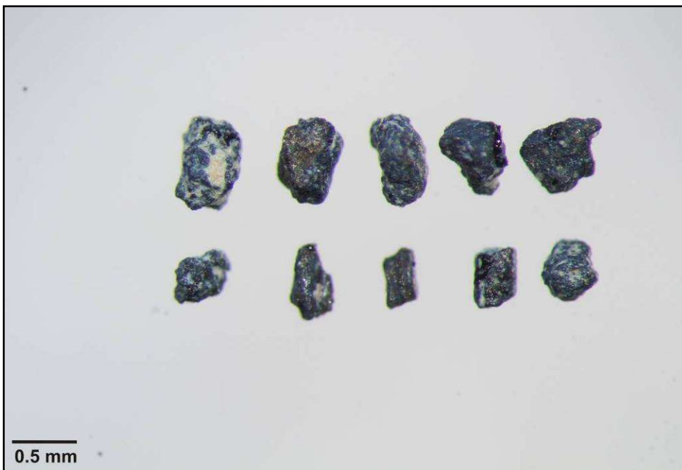
Figure C.24 Covellite grains from the 0.25-0.5mm fraction from sample AR-16-224 belonging to core VTH2014-11.
