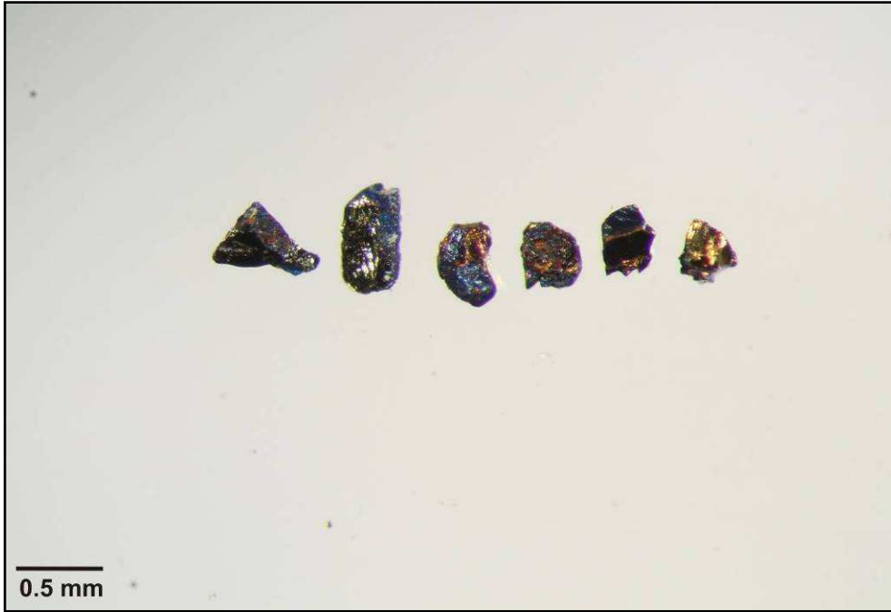
Figure C.40 Chalcopyrite grains from the 0.25-0.5mm fraction from sample AR-16-290 belonging to core JA16-001.
