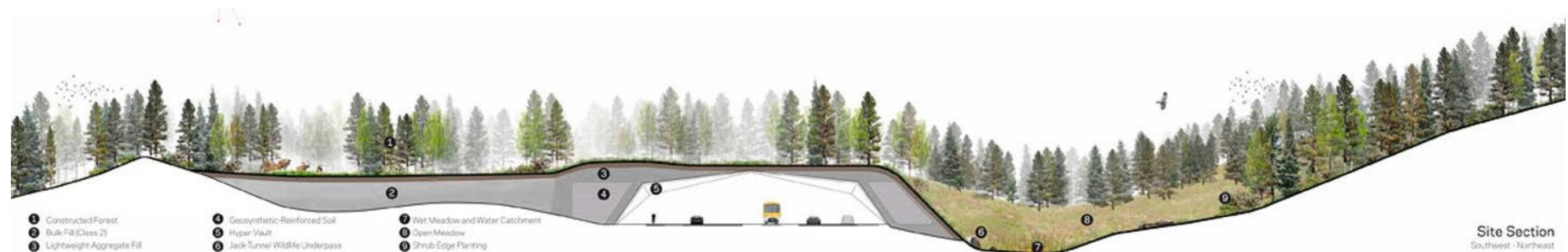
Fig 2.19 Hyper-Nature crossing, proposed site section showing shared animal and human zones.
