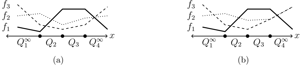
Figure 4.1: f_k 's and Q_r 's for an example 3-class ReLU classifier where the input x \in \mathbb{R} . Q_1^\infty and Q_4^\infty are infinity polytopes. (a) For sufficiently large (small) x , there is a unique k^* = 1 in Q_4^\infty ( k^* = 1 in Q_1^\infty ). (b) For sufficiently large x , there are multiple k^* 's in Q_4^\infty ( k^* = \{2, 3\} ). For sufficiently small x , there is a unique k^* = 3 in Q_1^\infty .
