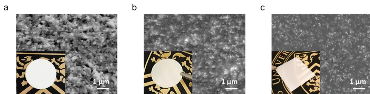
Figure 5.5 SEM and optical images (insets) of (a) LAGP pellet, (b) PL membrane and (c) PLE membrane with 30% EMITFSI. Reproduced with permission from J. Electrochem. Soc. , 166, H205 (2019). Copyright 2019, The Electrochemical Society [110].
