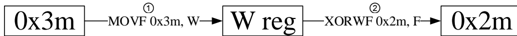
Figure 4.16: Instructions used in ARK_i of software implementation of AES, m \in [0 : F]
