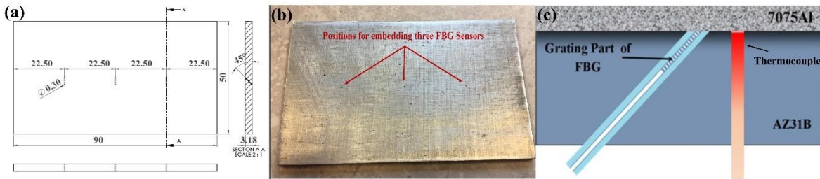
Fig B. 1: a) Sample drawing and geometry of AZ31-H24 (all dimensions in mm); b) Position of FBG sensors; c) schematic of grating position and a thermocouple.
