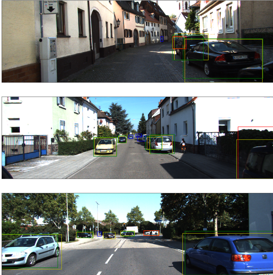
Figure 1.2: Example of FN car detections. Red boxes are FN car detections, yellow boxes are the ground truth annotations, green boxes are TP car detections, and blue boxes are unlabelled image regions of the “Don’t Care” class in KITTI. In these samples, the object detection network initially proposed that the red boxes were objects, but discarded them in the later layers by classifying them as background. Any cars that were detected by the model in the Don’t Care regions are not shown.
