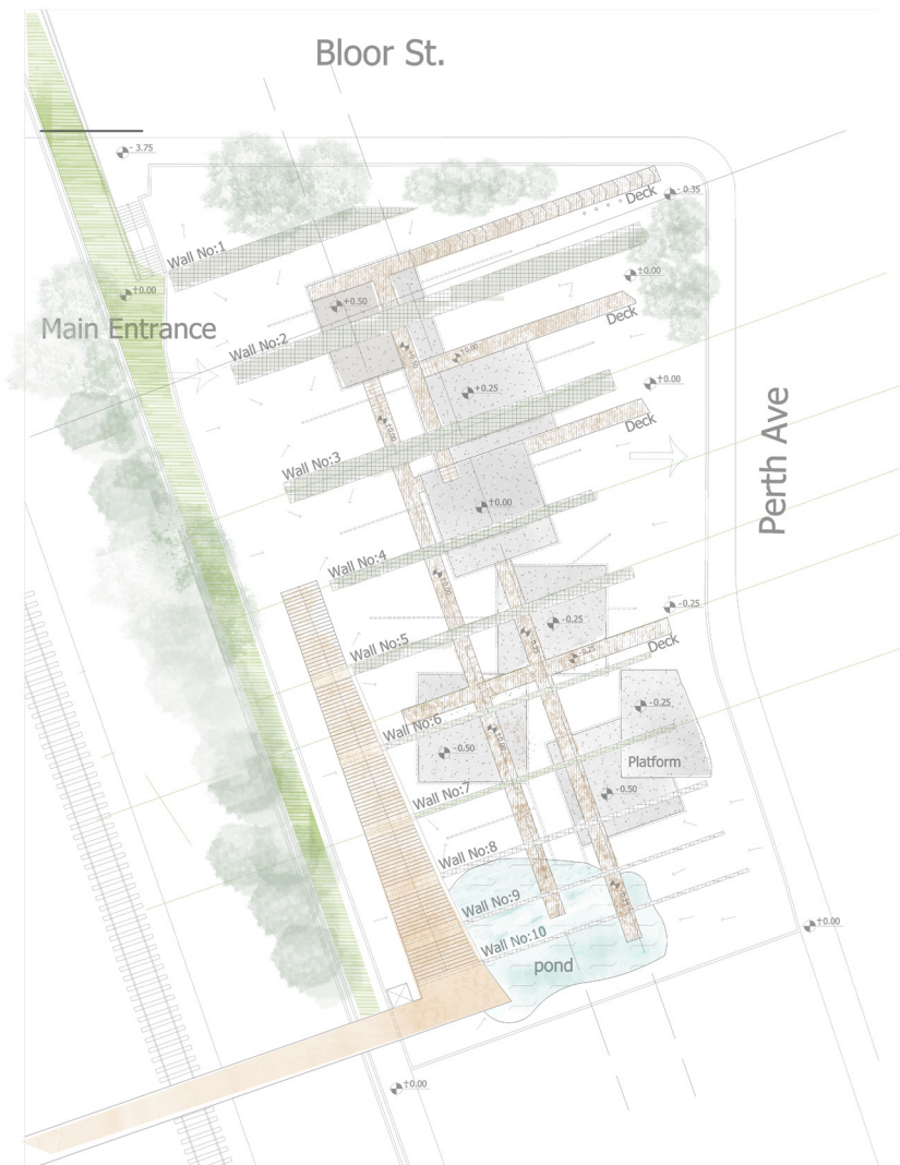
Fig 46. Site Plan – Organization of event Platforms, pedestrian pathway, bridge, pond, and green rooms
