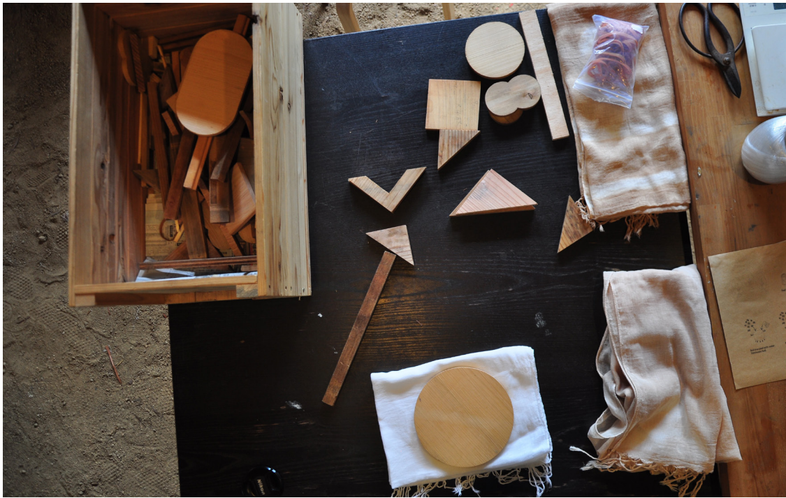
Figure 3.14: The process of making a scarf using the “itajime-shibori” technique. Here the wooden blocks are about to be clamped to the cotton cloth, which will create the pattern on the textile.
