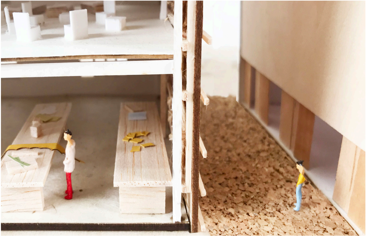
Figure 4.19: New pathways between split volumes, and a sectional portion showing the rice plant wall assembly of the daycare structure
