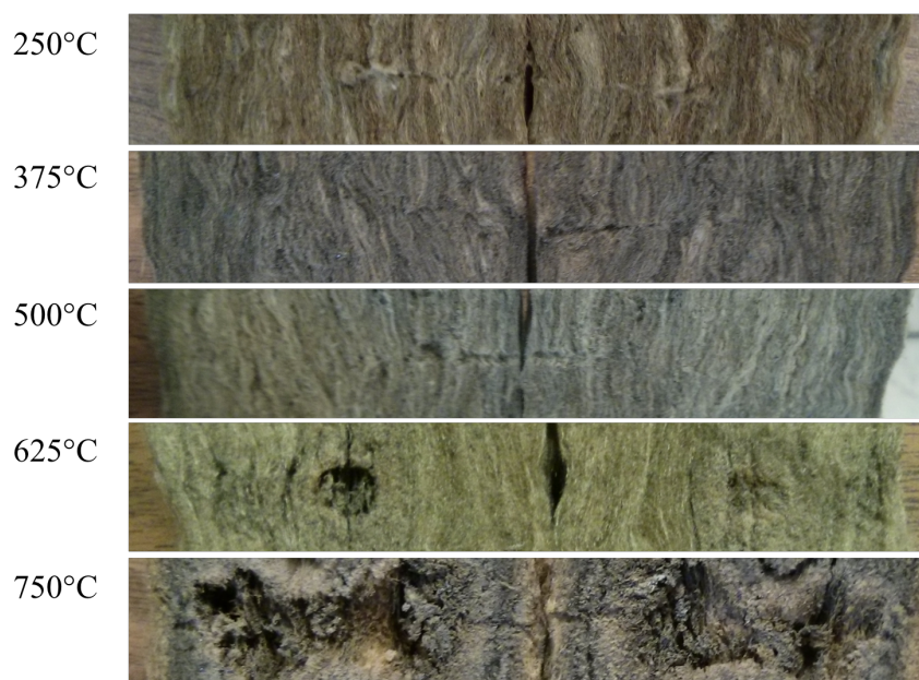
Figure 4.4: Interior Degradation of Tube Furnace Specimens.
