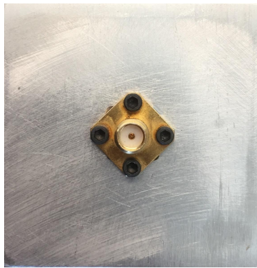
Figure 3.8: A coaxial line used to measure the permittivity of liquids. (a) An aluminum cube with a 3.6 cm deep hole as the outer layer with two 50\ \Omega connectors as the inners, each is 1.8 cm long. (b) Top view of the fabricated coaxial line filled with a MUT.
