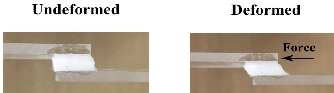
Figure 6. 3. The loading configuration for the shear relaxation tests: the cuboid was subjected to 50 % shear strain and left to relax for 300 seconds.
