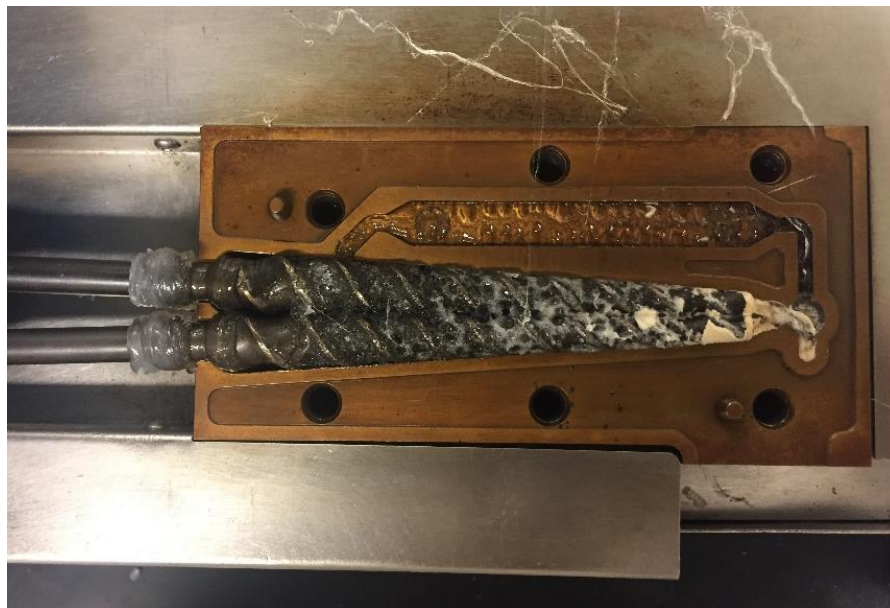
Figure 50: Obstruction of the extruder by the dry cellulose and PP mixture.
