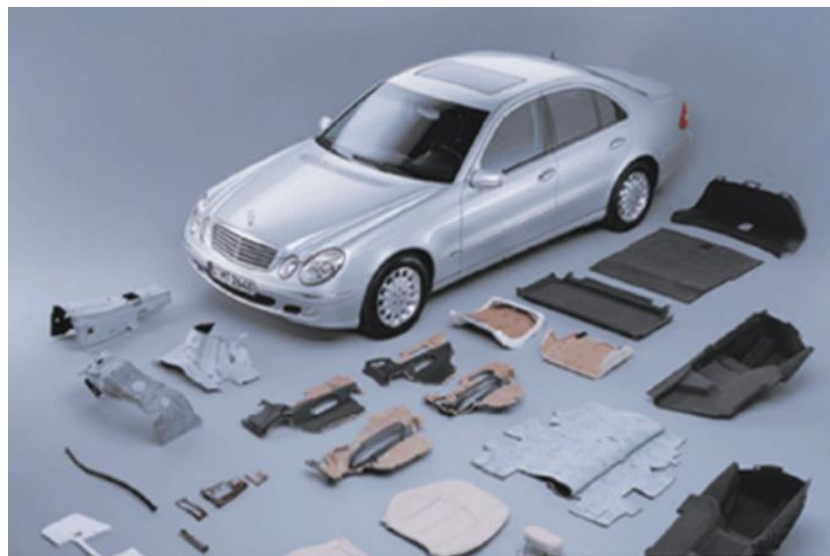
Figure 2: Automobile components made of natural fiber composites [2], under the Creative Commons Attribution License.
